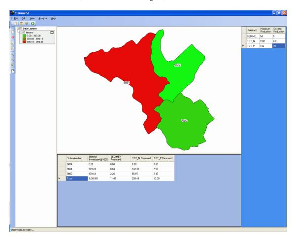
More investments in BMP technology are required, both in subwatershed 9664 and 9802. Also, the amounts of SEDIMENT and TOT\_N removed also increase because the BMP's installed to remove phosphorous also typically remove sediment and nitrogen.
