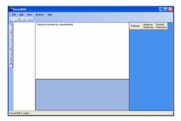
An array of menu options and tool bar shortcuts is provided along the top. Along the left is a tool strip for the GIS displays. Using File/Add GIS Layer, or clicking on the Add Layer tool allows the user to navigate to the location of a GIS "shape" file containing a map of the drainage areas. The three drainage analysis from the "Tacony" example is shown below.
