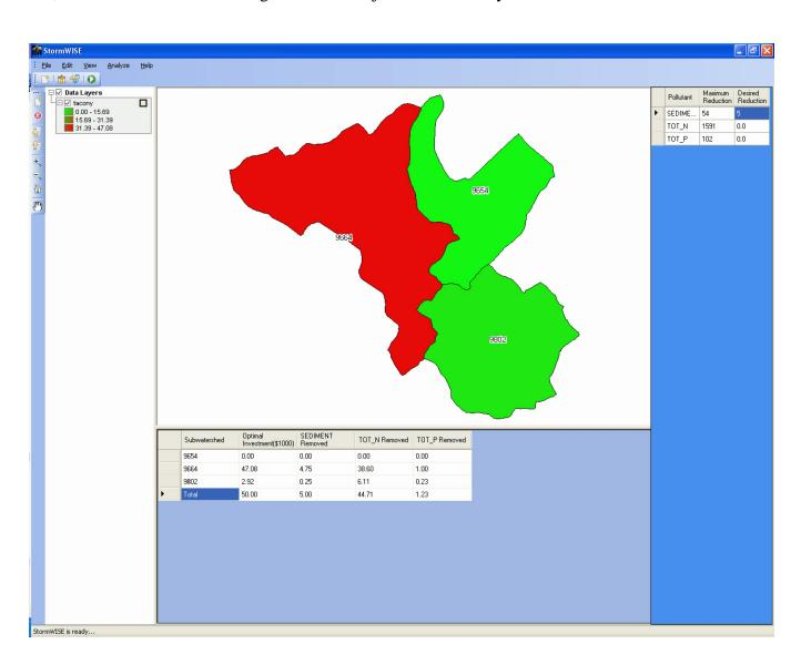
Note that the solution above yields very little of the potential 102 pounds annually of phosphorous removal. If the user now enters the amount of 10 in the Desired Reduction column for TOTAL\_P, and runs the model again, the result is shown below.
